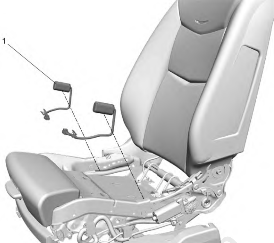
Fig. 5: Front Seat Lane Departure Warning Actuator
